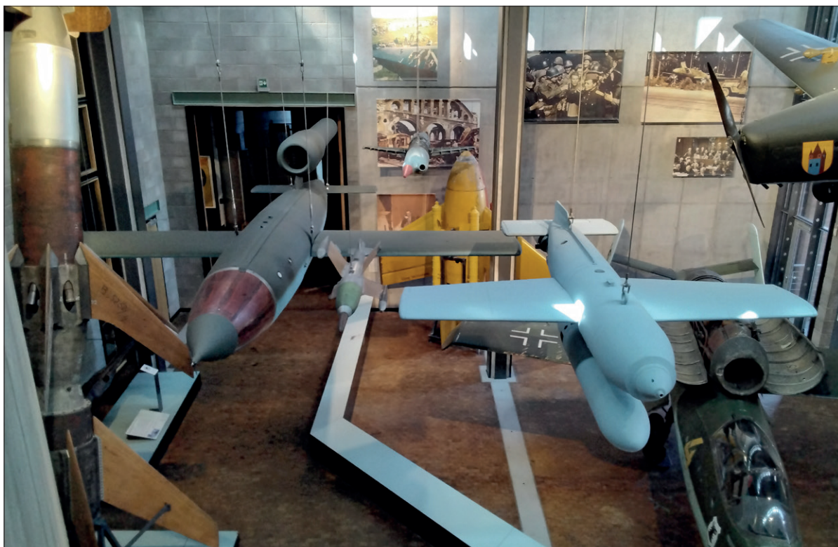
Rocket technology of the Third Reich. A Rheintochter anti-aircraft missile on the left, a V1 early cruise missile on the right, a smaller X-4 air-air missile next to it and an Hs 293 on the far right. A Smetterling missile hangs in the background and a yellow-painted Enzian missile sits on the floor. [Photo: Petr Uzsák]
