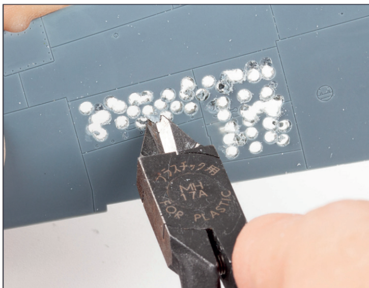
I'll connect the small holes to form a larger one using pliers.
