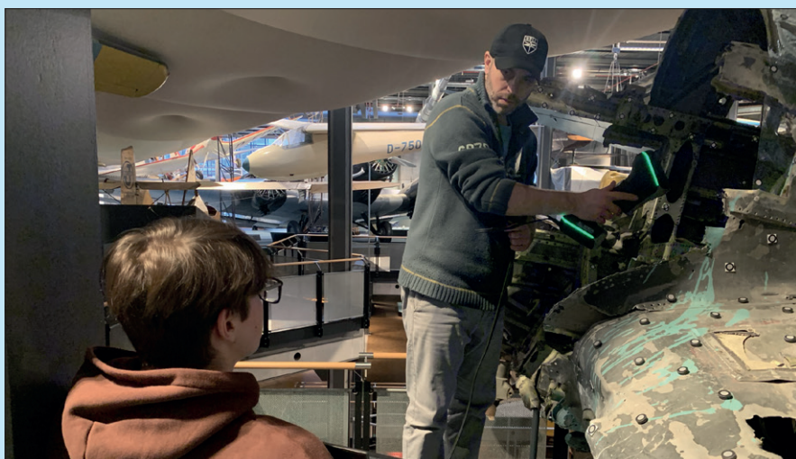
When scanning, dozens of registration marks must be applied to the scanned surface. These are either magnetic or electrostatic, and do not disturb the surface of the exhibit in any way.
