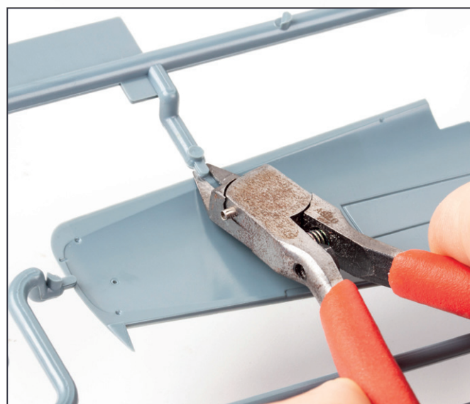
At the beginning of this article, I'd like to recap the basics from the last one—using single-blade pliers to remove parts from the wing halves. I detach the bottom sprues by laying the blade face of the pliers flush with the wing surface.
