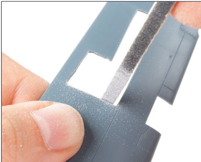
And sand the necessary areas with a finer file.
