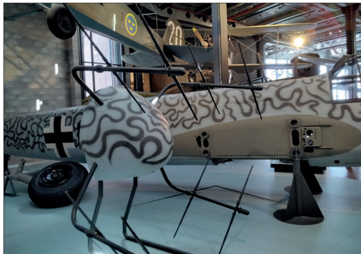
Ju 88G nose with FuG 220 radar antenna dipoles. [Photo: Petr Uzsák]
