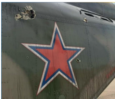
A Russian Mi-8AMTSh helicopter damaged by shrapnel from an air-defense missile.
