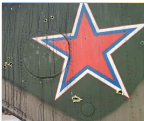
A Russian Mi-8AMTSh helicopter damaged by shrapnel from an air-defense missile.
