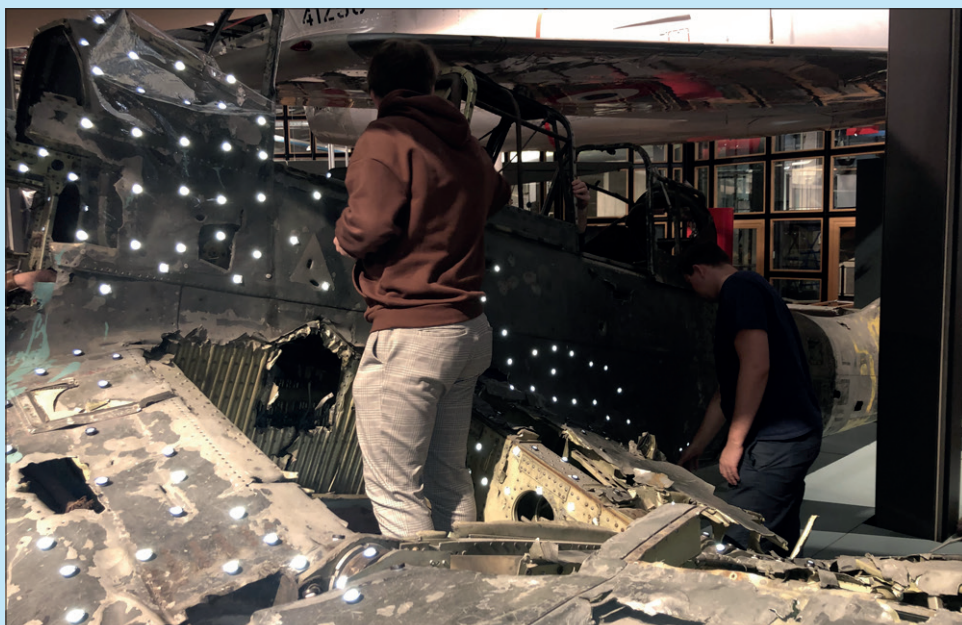
When scanning, dozens of registration marks must be applied to the scanned surface. These are either magnetic or electrostatic, and do not disturb the surface of the exhibit in any way.
