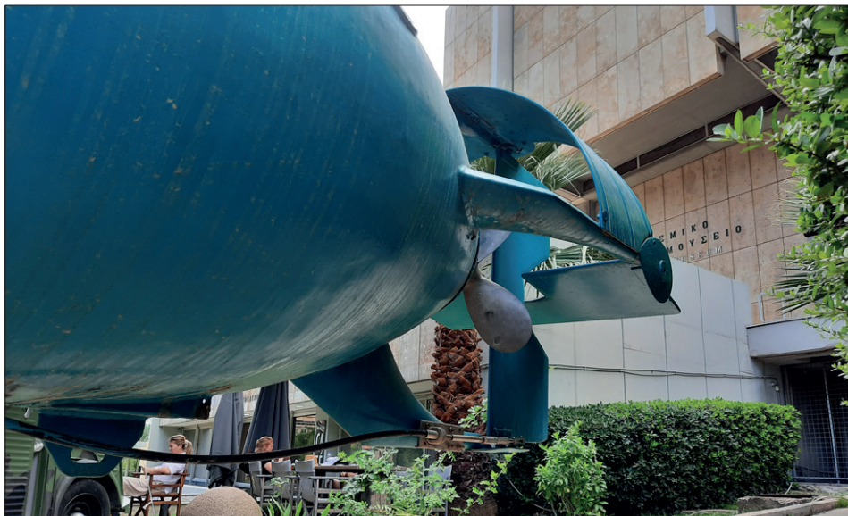
Detail of the rear of the CE2F/X60 mini-submarine, with the propeller and control surfaces clearly visible.
