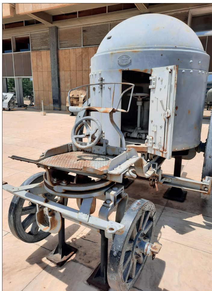
The front part of a Krupp-Schuman vehicle. The driver's seat and the mechanism for closing the turret hatch are worth noting.
